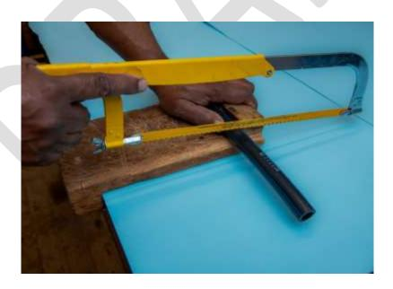
Safety measure • Ensure that the blade is properly tightened before cutting.
