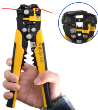
Using an automatic stripper to strip a wire
